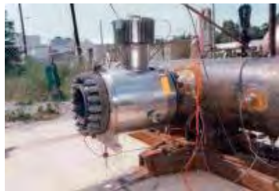
Depressurization Valve test
